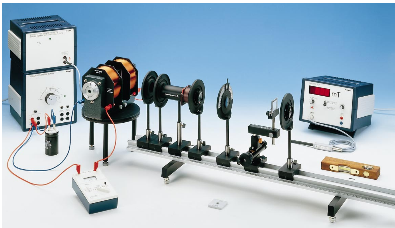
Fig.1: Experimental set-up for the Zeeman effect.
